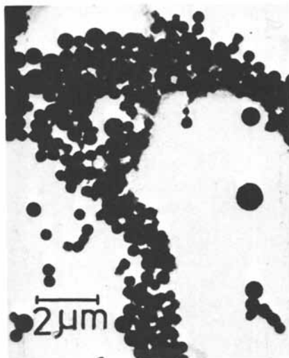
Figure 16. Electron micrograph of monomer emulsion of Figure 15 after 23 hr of stirring at 60°C and 600 rpm
