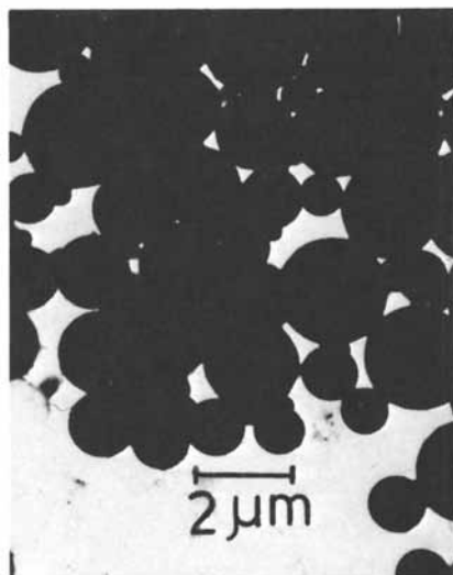
Figure 14. Electron micrograph of monomer emulsion of Figure 13 after 21 hr stirring at 60°C and 600 rpm
